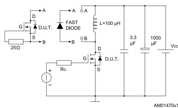
**Figure 17: Unclamped inductive load test circuit**
