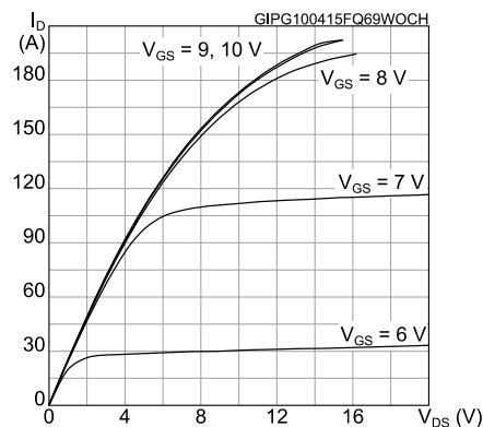
Figure 5: Transfer characteristics
