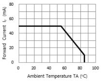
Fig. 3 FORWARD CURRENT VS. DERATING CURVE
