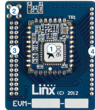
Figure 3: HumPRC™ Series Transceiver Carrier Board
