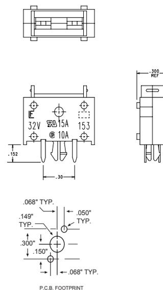
**PCB MOUNT FUSE HOLDER FOR MINI® STYLE BLADE FUSE**
