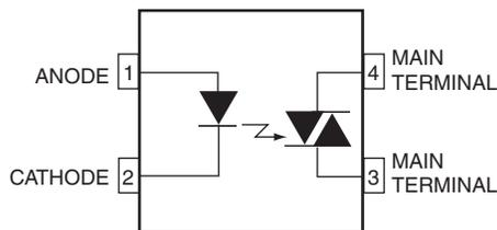
Figure 1. Functional Schematic
