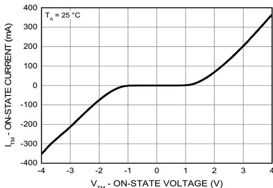
Fig 9. On-State Characteristics
