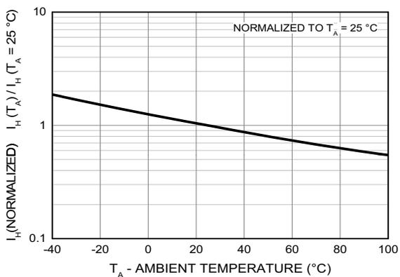
Fig 5. Normalized Holding Current vs. Ambient Temperature
