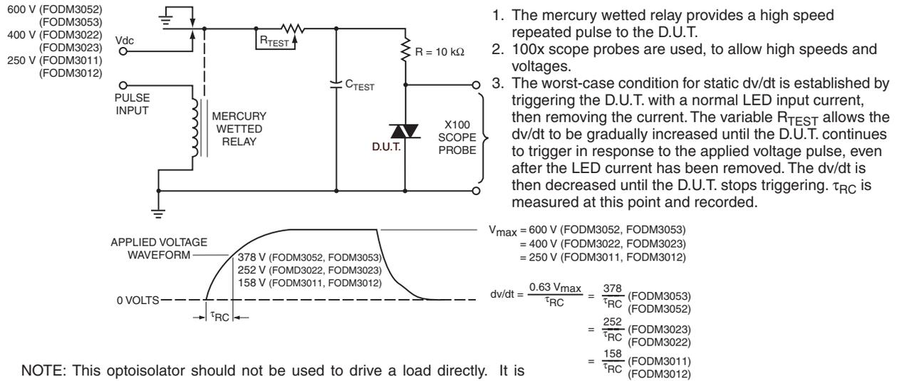
NOTE: This optoisolator should not be used to drive a load directly. It is intended to be a trigger device only.
