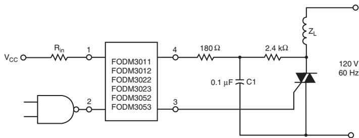
Figure 12. Inductive Load with Sensitive Gate Triac (I<sub>GT</sub> ≤ 15 mA)
