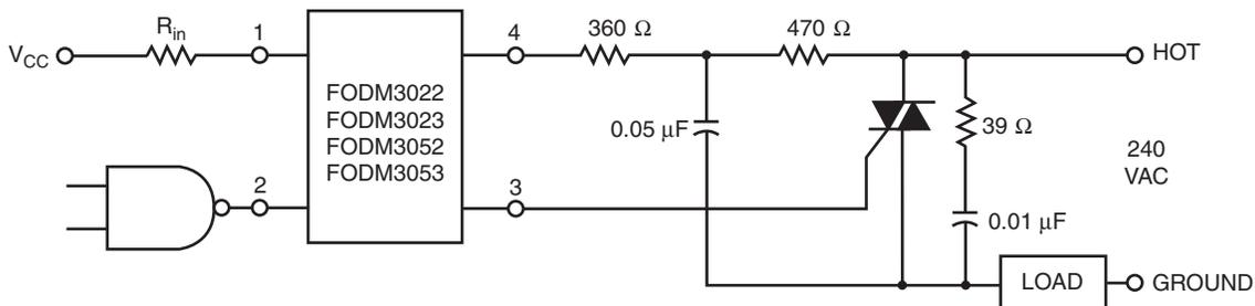
In this circuit the “hot” side of the line is switched and the load connected to the cold or ground side.
