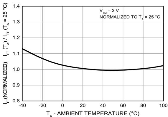
Fig 6. Normalized Trigger Current vs. Ambient Temperature
