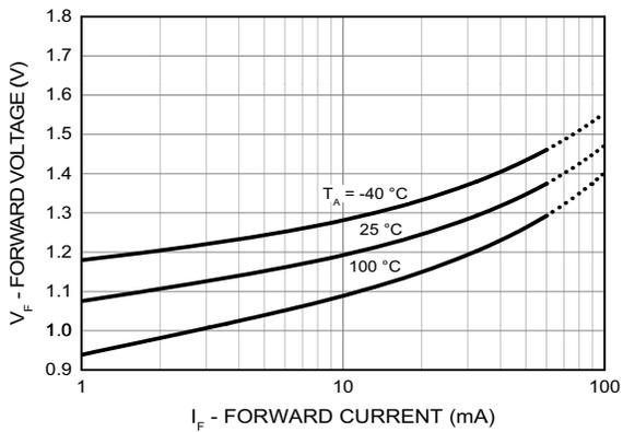
Fig 3. LED Forward Voltage vs. Forward Current
