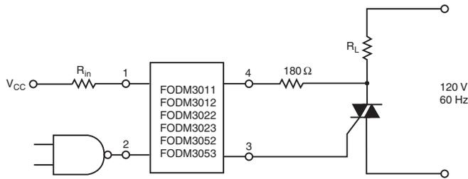
Figure 11. Resistive Load
