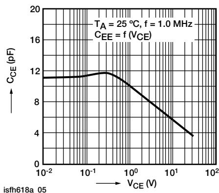
Fig. 8 - Transistor Capacitance
