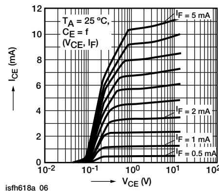
Fig. 9 - Output Characteristics
