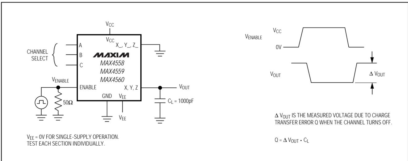
Figure 3. Charge Injection
