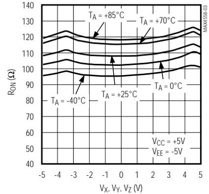
**ON-RESISTANCE vs.  $V_X, V_Y, V_Z$  AND TEMPERATURE (SINGLE SUPPLY)**
