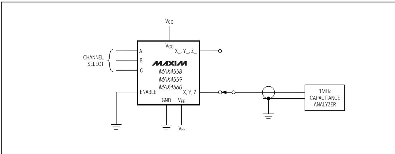
Figure 5. Channel Off/On-Capacitance
