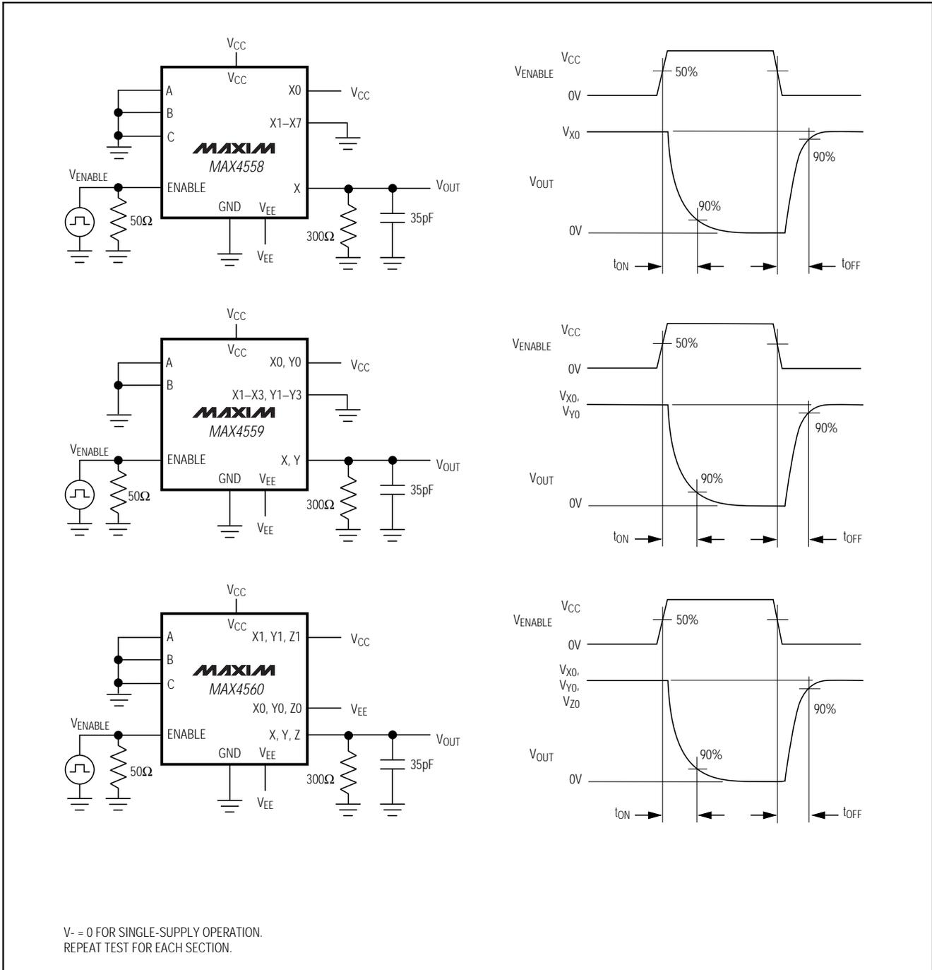
Figure 1. Switching Times
