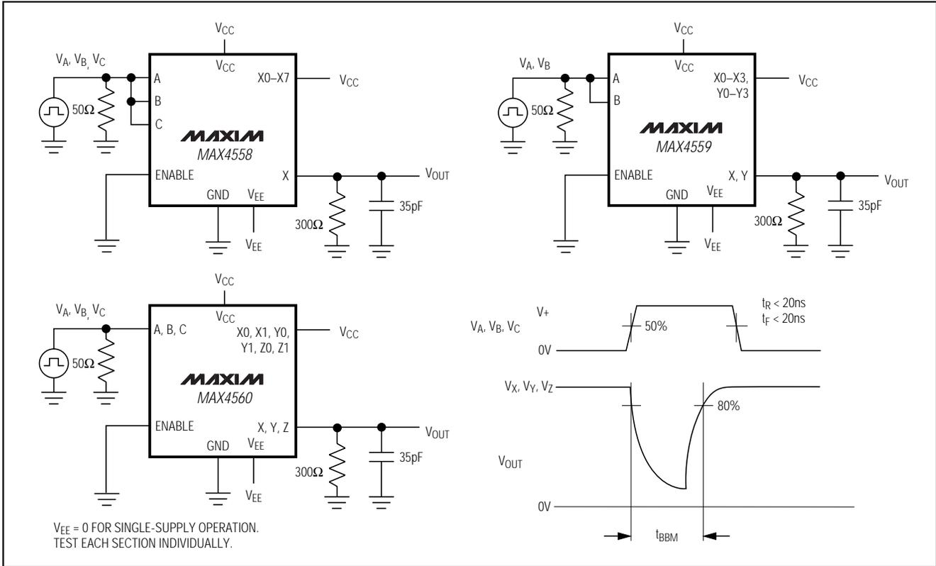
Figure 2. Break-Before-Make Interval
