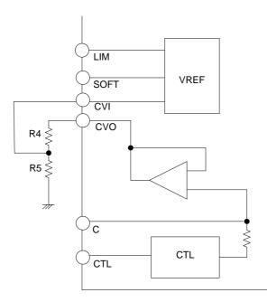
(2) Movement along the Y-axis (resistance divided between CVO and  $V_{CC}$ )
