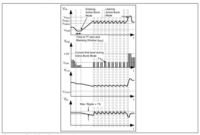
Figure 9 **Signals in Active Burst Mode**
