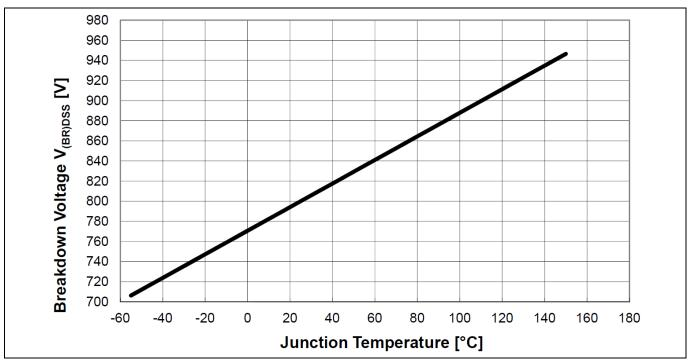
Figure 12 Drain-source breakdown voltage;  $V_{BR(DSS)}=f(T_j)$ ,  $I_D=0.25mA$
