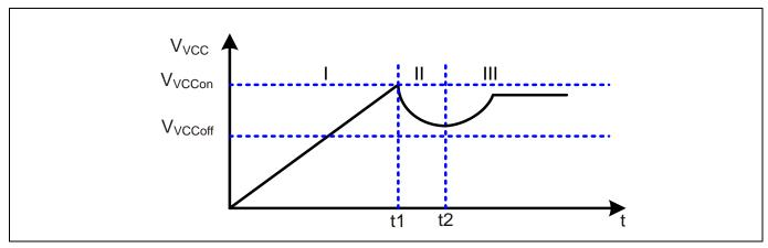
Figure 4 VCC voltage at start up
