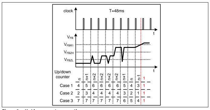
Figure 6 Up/down counter operation
