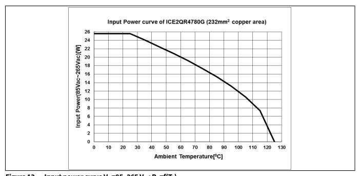
Figure 13 Input power curve V<sub>IN</sub>=85~265 V<sub>AC</sub>; P<sub>in</sub>=f(T<sub>a</sub>)
