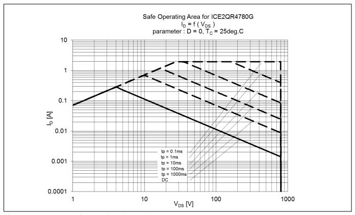
Figure 10 Safe Operating Area (SOA) curve for ICE2QR4780G
