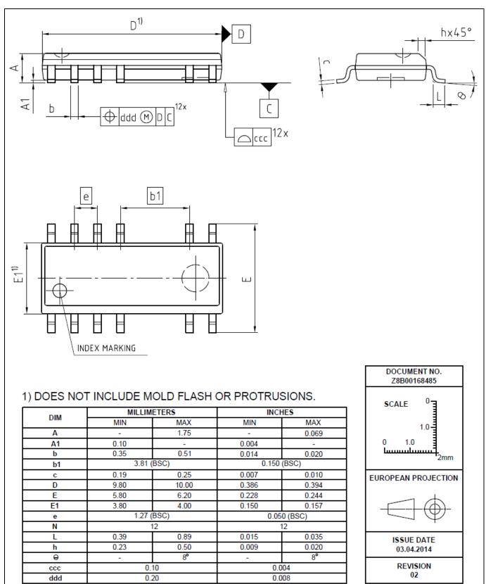
Figure 15 PG-DSO-12 (Pb-free lead plating Plastic Dual-in-Line Outline)
