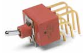
E301MD1AV2BE Vertical Actuation 3PDT
