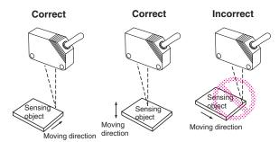
Install the Sensor as shown in the following illustration if each sensing object greatly differs in color or material.
