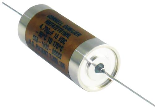
Type HHT has long life and rugged construction for high temperature environments. HHT capacitors are rated for full operating voltage at 175 °C and tested to 2000 hrs at rated voltage and temperature. 5000 hours of life at 150 °C with ripple current ratings up to 10 Arms.
