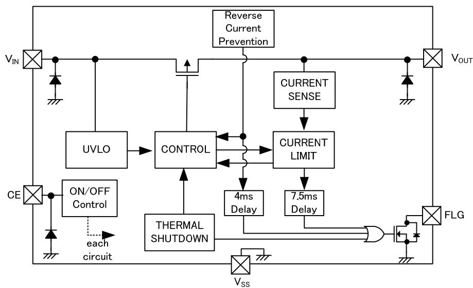
\* Diodes inside the circuit are an ESD protection diode and a parasitic diode.
