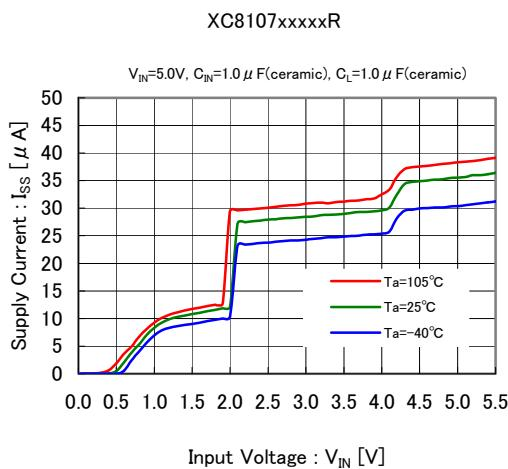
(7) Supply Current vs. Ambient Temperature
