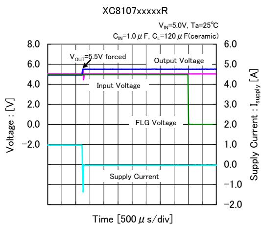
(40) Reverse Voltage Released Voltage ( $C_L=120 \mu F$ )
