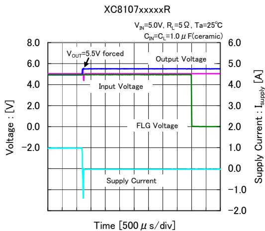
(38) Reverse Voltage Released Voltage ( $C_L=1.0 \mu F$ )
