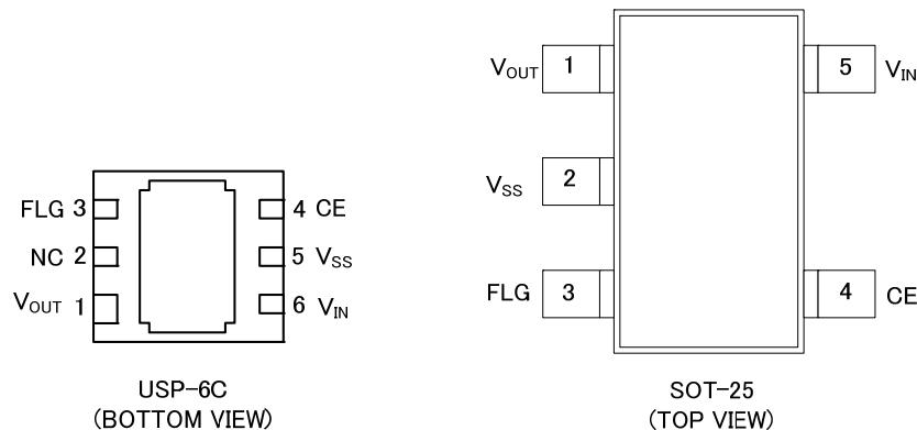
\* The dissipation pad for the USP-6C packages should be solder-plated for mounting strength and heat dissipation.
