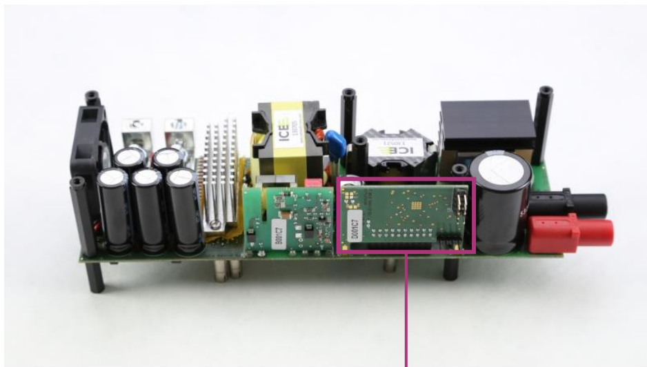
Digital control card: KIT_600W_LLC_DI_CTRL
