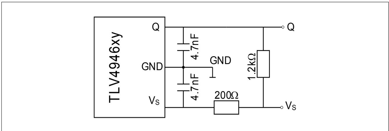
**Figure 5 Application circuit**
