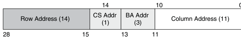
Figure 2-8. Mapped Address for the Example
