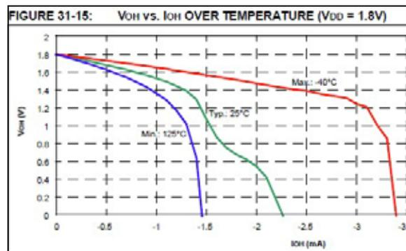
FIGURE 8-2: Example PIC<sup>®</sup> Microcontroller  $V_{OH}$  Characterization Graph ( $V_{DD} = 1.8V$ ).
