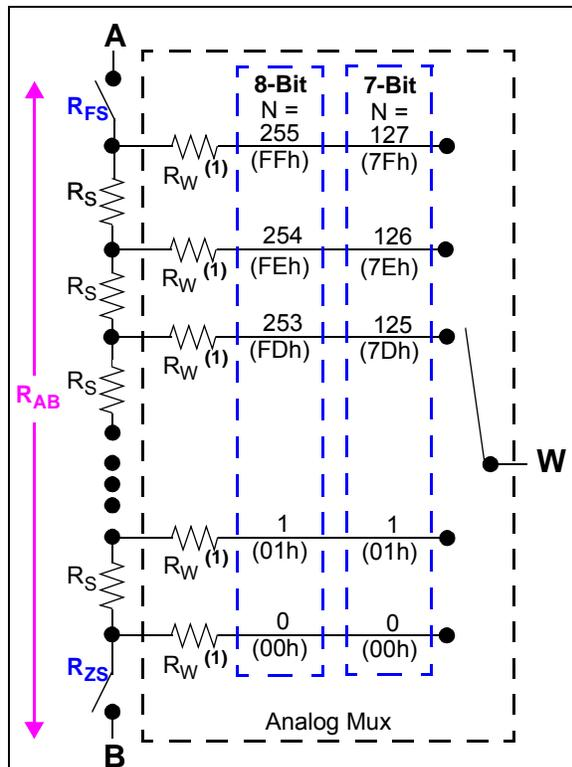
**Note 1:** The wiper resistance is dependent on several factors including wiper code, device V+ voltage, terminal voltages (on A, B and W), and temperature. Also for the same conditions, each tap selection resistance has a small variation. This  $R_W$  variation has greater effect on some specifications (such as INL) for the smaller resistance devices (5.0 k $\Omega$ ) compared to larger resistance devices (100.0 k $\Omega$ ).
