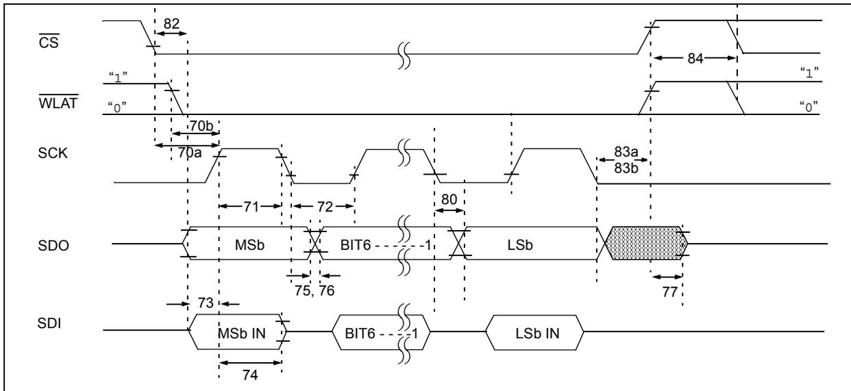
**FIGURE 1-3: SPI Timing Waveform (Mode = 00).**
