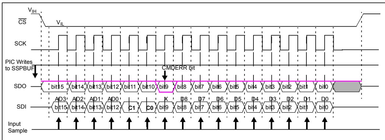
**FIGURE 6-3:** 16-Bit Commands (Write, Read) – SPI Waveform (Mode 0,0).
