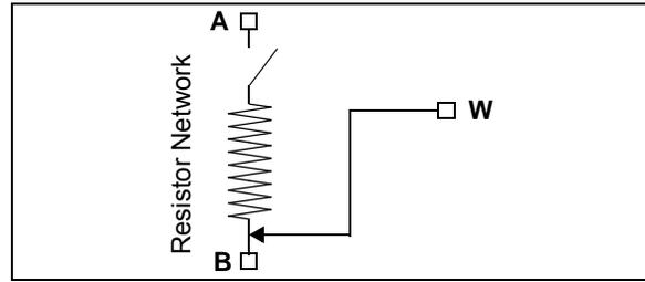
**FIGURE 5-11:** Resistor Network Shutdown State ( $R0HW = 0$ ).
