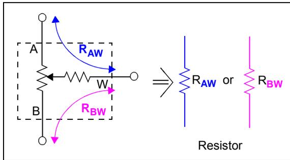
**FIGURE 5-8:** Rheostat Configuration.
