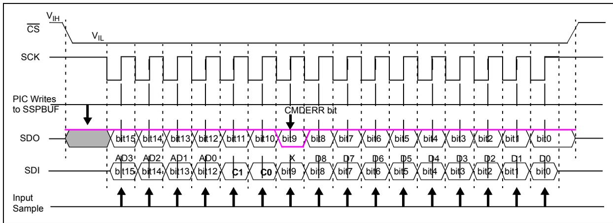
**FIGURE 6-2:** 16-Bit Commands (Write, Read) – SPI Waveform (Mode 1,1).
