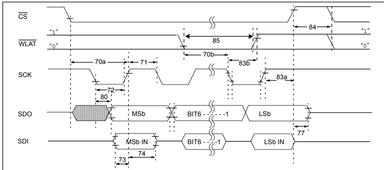
**FIGURE 1-2:** SPI Timing Waveform (Mode = 11).
