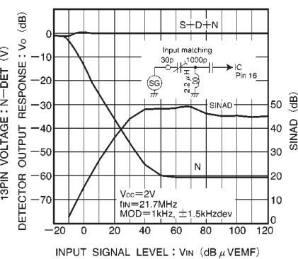
Fig. 15 Detector output response,
