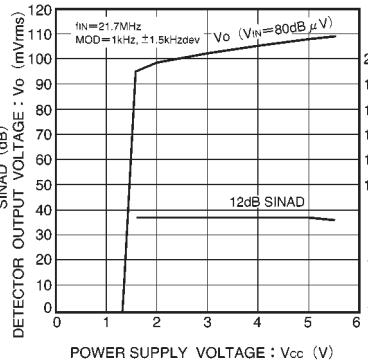
Fig. 8 Detector output voltage,
