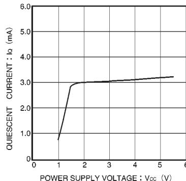
Fig. 4 Quiescent current vs. power supply voltage
