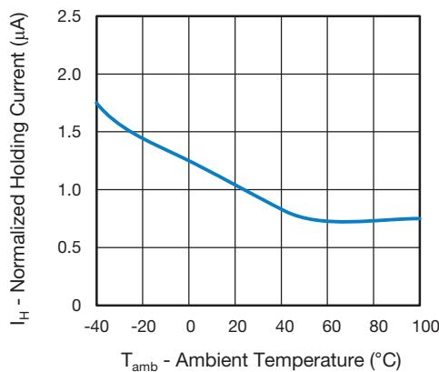
Fig. 9 - Normalized Holding Current vs. Ambient Temperature
