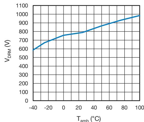
Fig. 14 - Peak Off-State Voltage vs. Ambient Temperature
