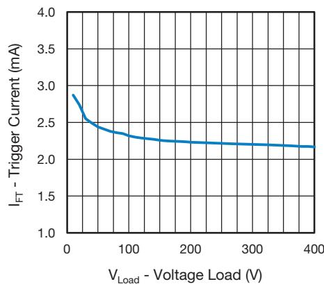
Fig. 12 - Trigger Current vs. Voltage Load
