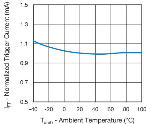
Fig. 7 - Normalized Trigger Current vs. Ambient Temperature
