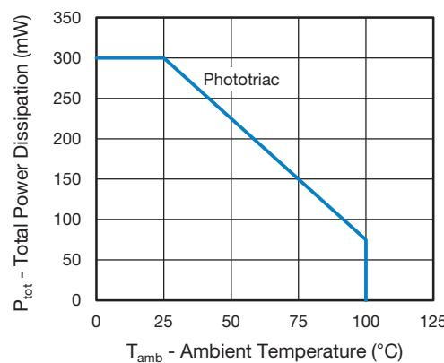
Fig. 2 - Total Power Dissipation vs. Ambient Temperature (Phototriac)
