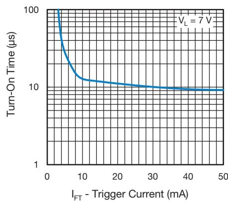
Fig. 8 - Turn-On Time vs. Trigger Current
