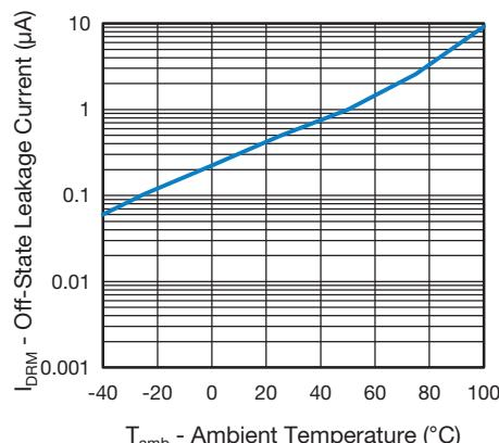
Fig. 6 - Off-State Leakage Current vs. Ambient Temperature
