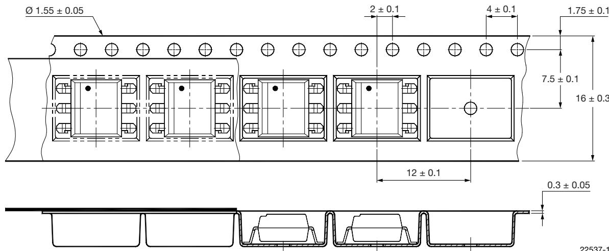
Fig. 17 - Tape and Reel Drawing, 1000 Units per Reel
