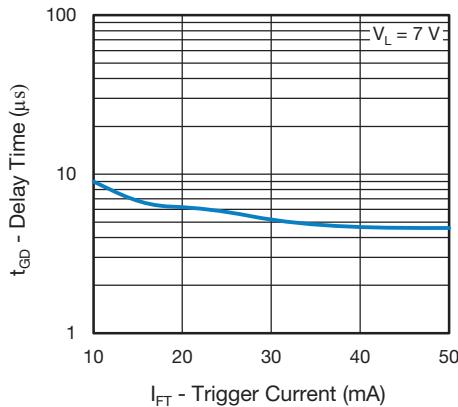
Fig. 10 - Delay Time vs. Trigger Current
