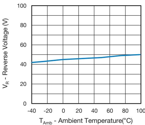
Fig. 4 - Reverse Voltage vs. Ambient Temperature
