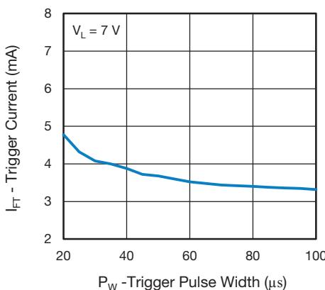
Fig. 11 - Trigger Current vs. Trigger Pulse Width
