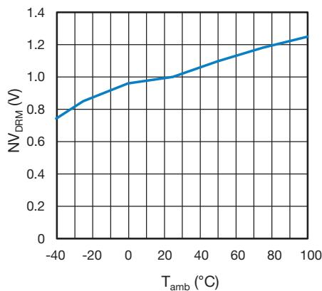
Fig. 15 - Normalized Off-State Voltage M2/M1 vs.
