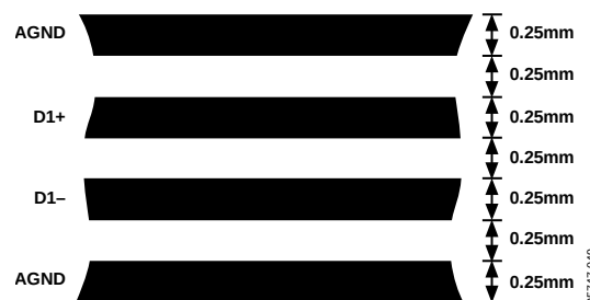
Figure 61. Arrangement of Signal Tracks
