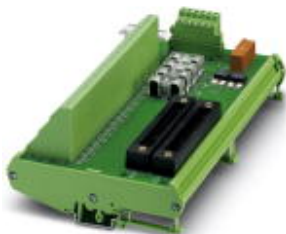
32-channel digital input module with screw connection and redundant voltage supply. Suitable for Yokogawa ADV151 and ADV161 cards.
