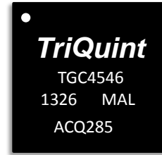
28-pin 5x5mm QFN package
