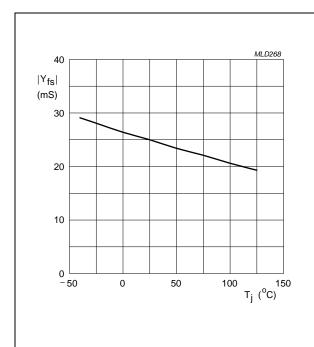
Forward transfer admittance as a function of junction temperature; typical values.
