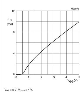
$R_{G1}$  = 120 k $\Omega$  (connected to  $V_{GG}$ );  $T_i$  = 25 °C.
