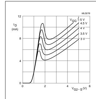
$V_{DS} = 5 \text{ V}; T_j = 25 \text{ }^{\circ}\text{C}.$  $R_G$  = 120 k $\Omega$  (connected to  $V_{GG}$ ).
