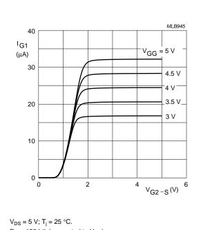
$R_G$  = 120 k $\Omega$  (connected to  $V_{GG}$ ).
