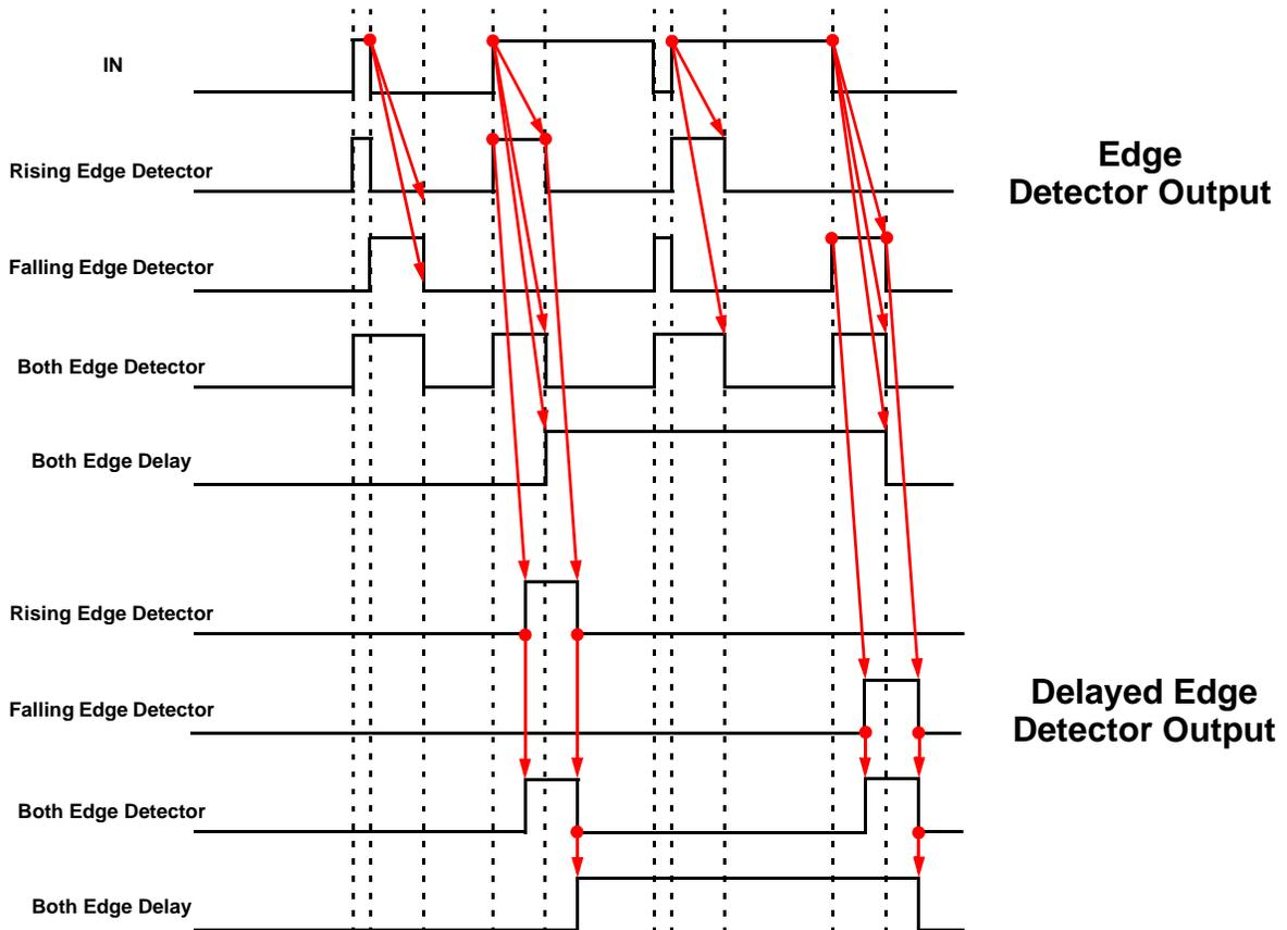
Figure 31. Glitch Filtering for Edge Detector Output
