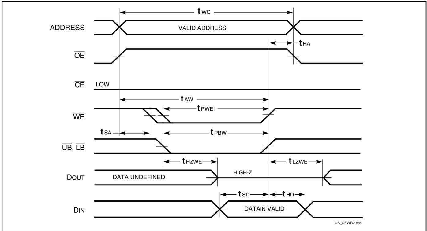
**WRITE CYCLE NO. 3** ( $\overline{OE}$  is LOW During Write Cycle) <sup>(1)</sup>
