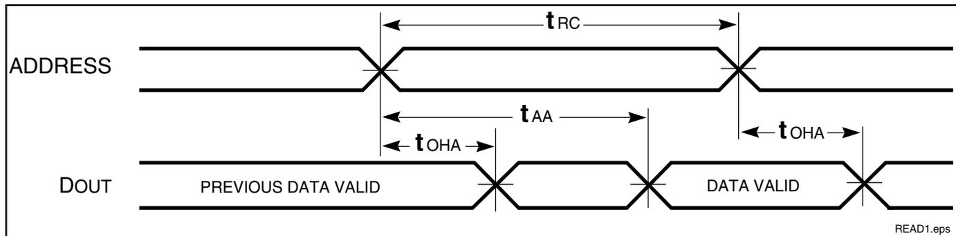
**READ CYCLE NO. 2<sup>(1,3)</sup>** ( $\overline{CE}$ ,  $\overline{OE}$  and  $\overline{UB/LB}$  Controlled)
