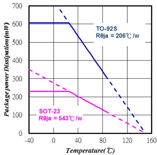
Figure 8. Temperature vs. Power Dissipation
