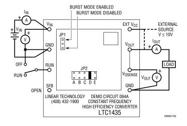
Figure 3. Proper Measurement Setup
