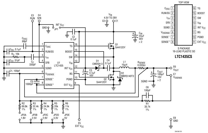
Figure 1. LTC1435 Constant Frequency, High Efficiency Converter
