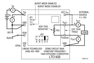
Figure 4. Remote Output Voltage Sense
