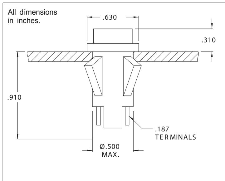
Mounting: Will snap-fit into Ø.500/.505 hole in panels .020/.100 thick. Push-on speednut SN0461 also available.
