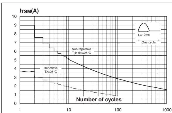
**Figure 14. Non repetitive surge peak on-state current for a sinusoidal pulse with width  $t_p < 10\text{ms}$ , and corresponding value of  $I^2t$**
