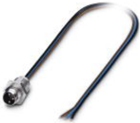
Sensor/actuator flush-type plug, 3-pos., M8, front/screw mounting, with M8 thread, with 0.5 m TPE litz wire, 3 x 0.25 mm 2
