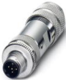
Bus system connector, male connector, straight, 5-pos., M12, shielded, gold-plated contacts, B-encoded, screw connection, metal knurl, PG11 cable gland
