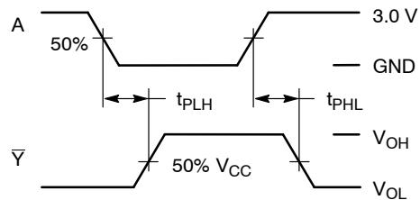
Figure 4. Switching Waveforms
