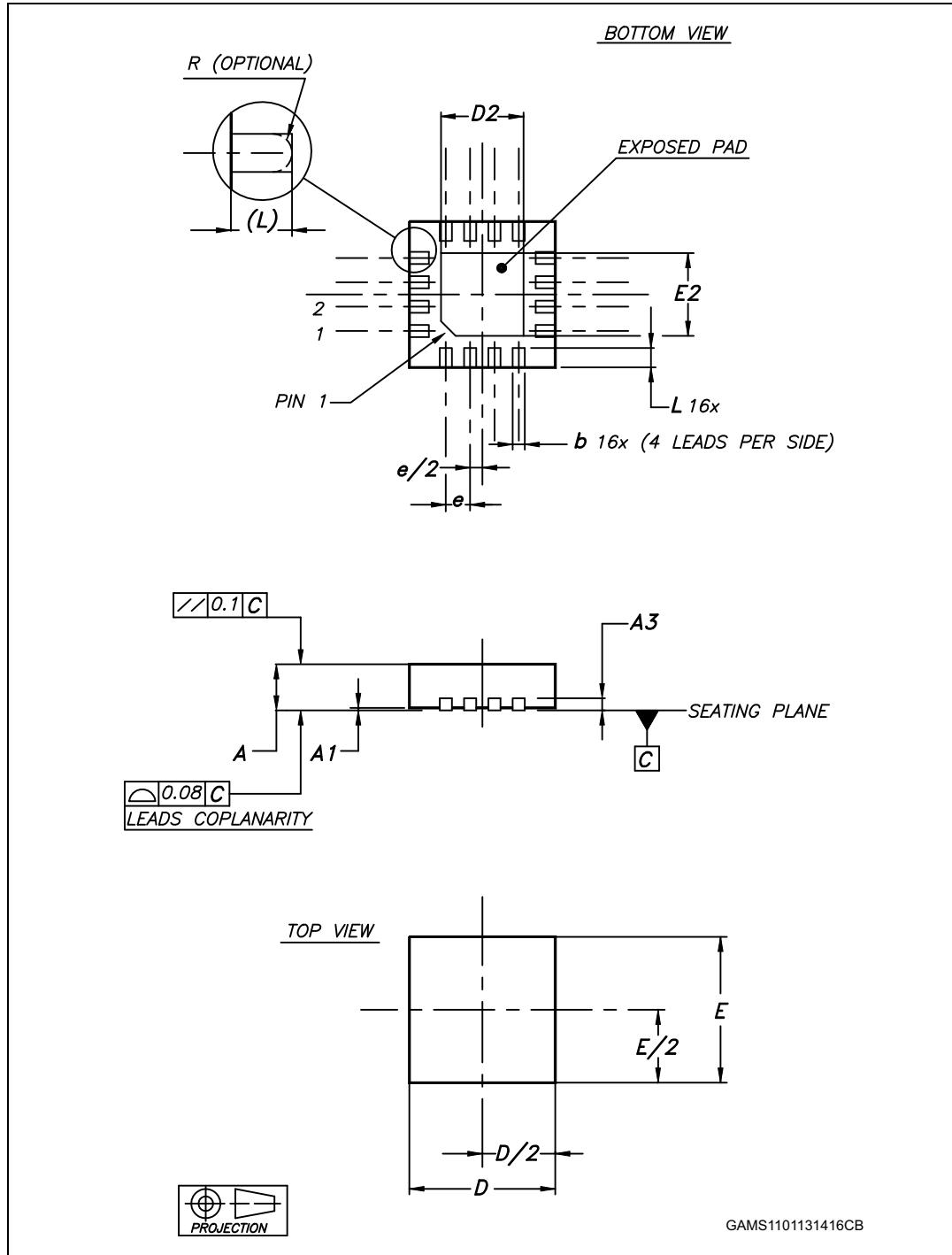
**Table 18. QFN16 3x3 mm package mechanical data (pitch 0.5 mm)**
