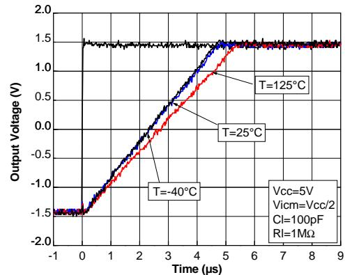
**Figure 16. Negative slew rate at  $V_{CC} = 5$  V with  $C_l = 100$  pF**
