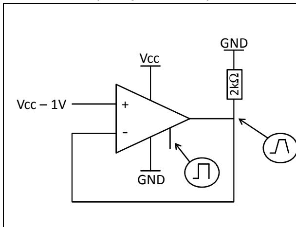
**Figure 23. Turn-on time,  $V_{CC} = 5$  V,
