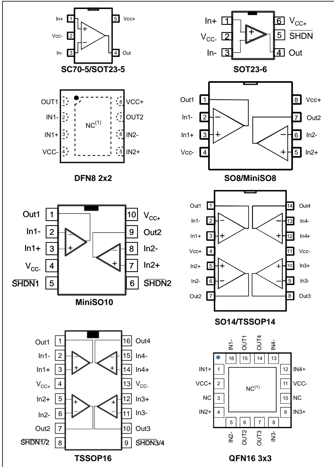
1. The exposed pads of the DFN8 2x2 and QFN16 3x3 can be connected to VCC- or left floating.
