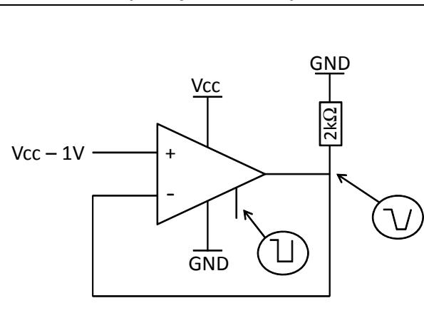
**Figure 24. Turn-off time,  $V_{CC} = 5$  V,
