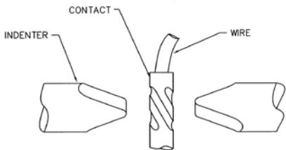
The model **SC8** has single flat-tipped indenters and accommodates wire sizes 12 thru 26 AWG. It accommodates the TP series positioners. It is 9 $\frac{3}{4}$ " in length and weighs approximately 15 oz. Gaging is accomplished with the G125 "GO/NO-GO" gage.
