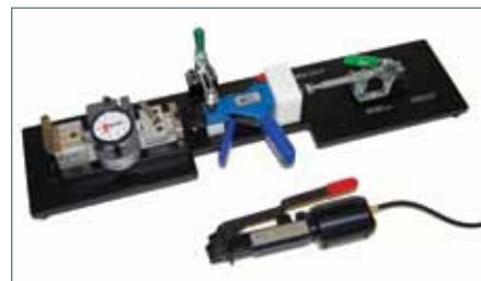
The **DBS-CG1-F** holding fixture secures the laboratory calibration instrument and banding tool in place during calibration. This fixture only works with the DBS-CG1 Calibration Instrument. (Banding tools and DBS-CG1 are sold separately.)
