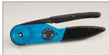
The **M300-25A** is designed for Pyle National Starline pin and socket contacts, **AWG sizes 10-18**. This tool is available in a pneumatic version, P/N WA27CL-25A.
