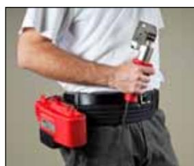
The battery and pump unit can be worn on a tool belt...
