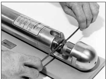
The DMC **ST825** Swaging Tool is used to swage terminals to flexible aircraft cable (usually stainless steel) and is built to meet government specifications. The complete tool consists of a cylinder and yoke assembly that is easily accessible for quick changing of dies, air hose assembly with a shut off valve and a single action foot control valve assembly with lubricator and air filter.
