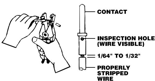
1. Determine the proper length of insulation to be removed. Wire must be visible in inspection hole. Insulation must be 1/64" – 1/32" from end of contact or inside of insulation cup.
