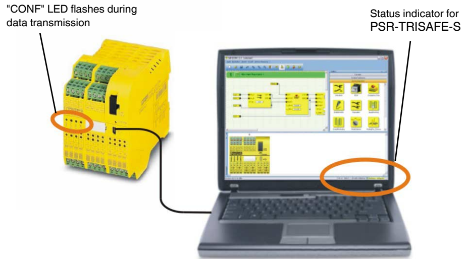
Figure 5-4 USB connection between PC and safety module
