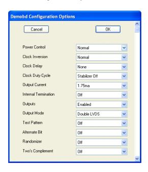
Figure 5. Demoboard Configuration Options
