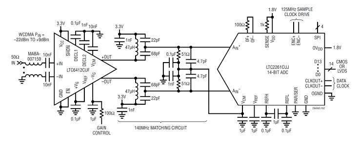
Figure 1. DC1600A Simplified Schematic
