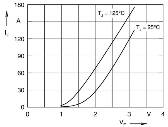
Fig. 4 Typ. forward characteristics of free wheeling diode
