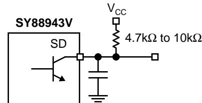
Figure 1. SD Output with Desired Rise Time
