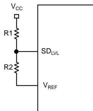
Figure 3. SD<sub>LVL</sub> Circuit
