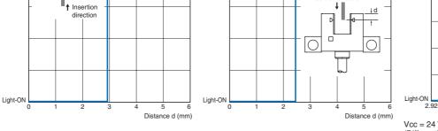
2.98 Distance d (mm) Vcc = 24 V, No. of repetitions: 20, Ta = 25°C (Differential travel = 0.025 mm max.)
