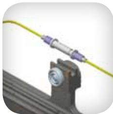
Complete Second Buffer Crimp and Remove Splice from Tool
