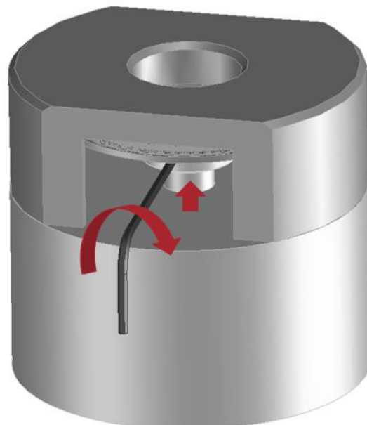
Figure 1d. Tighten the set screws
