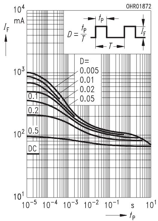
**Figure 5. Permissible Pulse Handling Capability,  $I_F = f(t_P)$ ,
