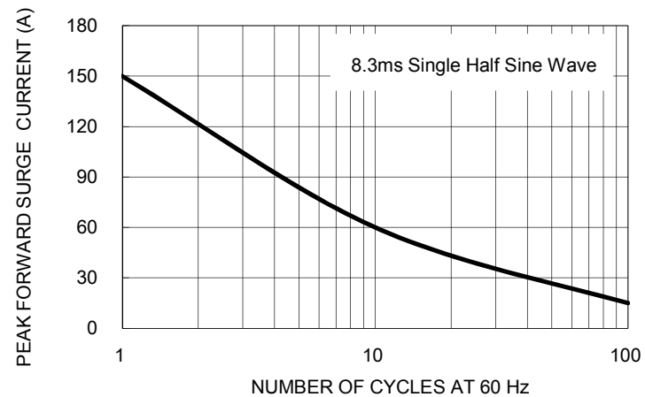
FIG. 2 MAXIMUM NON-REPETITIVE FORWARD SURGE CURRENT PER LEG
