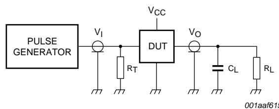
Test data is given in [Table 9](#). Definitions for test circuit:
