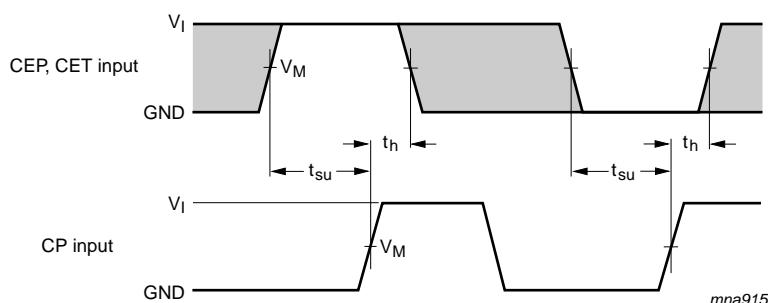
The shaded areas indicate when the input is permitted to change for predictable output performance.
