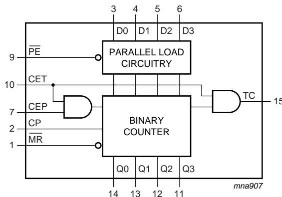
Fig 3. Functional diagram
