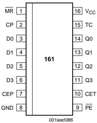
Fig 5. Pin configuration for SO16 and (T)SSOP16
