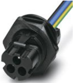
PRC device connector, black, 3-pos., 4 mm 2 /630 V/35 A, crimp connection, with 150 mm cable length, smoothly cut off at end
