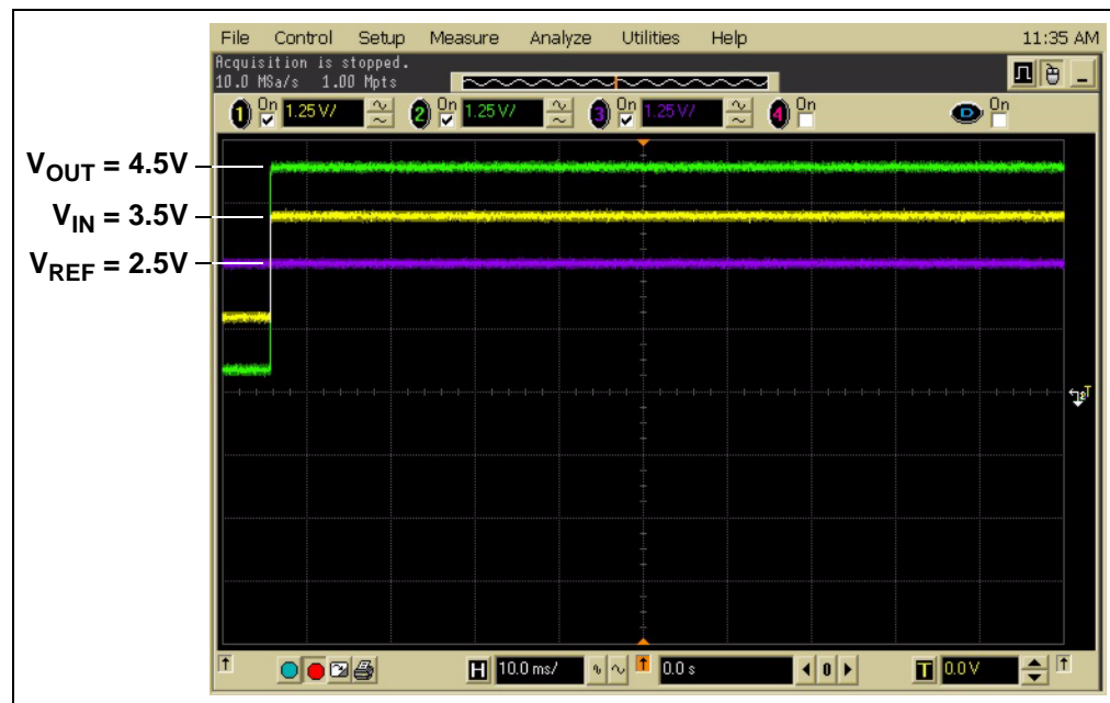
FIGURE 2-25: Measured Step Response.
