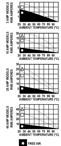
Mounted on a heat sink with 2 °C/watt rating
