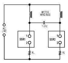
The resistors are unnecessary if the control circuit is designed to ensure that one SSR is off before the other SSR is on.
