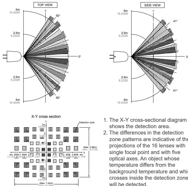
1. The X-Y cross-sectional diagram shows the detection area.
