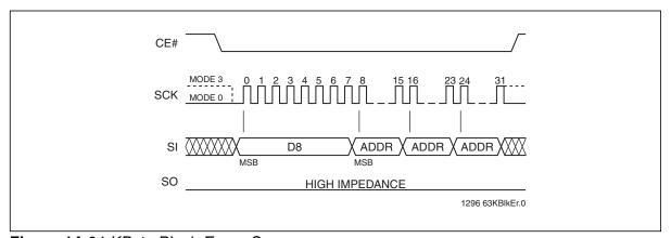
Figure 14:64-KByte Block-Erase Sequence
