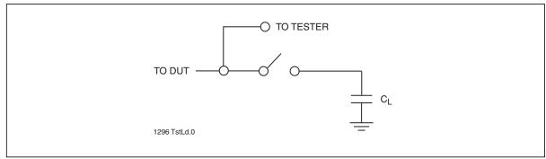
Figure 27:A Test Load Example
