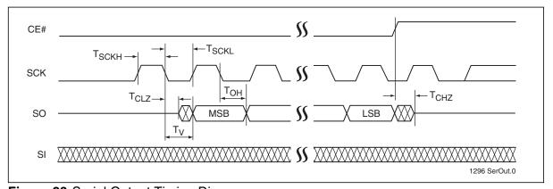
Figure 23: Serial Output Timing Diagram
