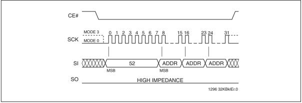
Figure 13:32-KByte Block-Erase Sequence
