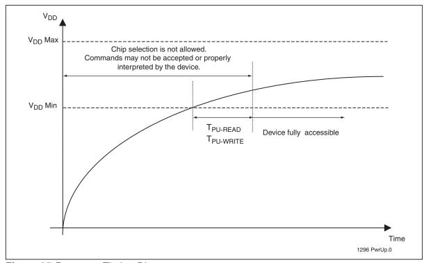
Figure 25: Power-up Timing Diagram
