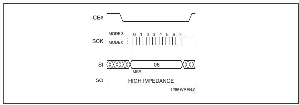
Figure 17: Write Enable (WREN) Sequence
