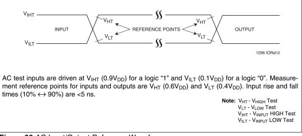
Figure 26:AC Input/Output Reference Waveforms
