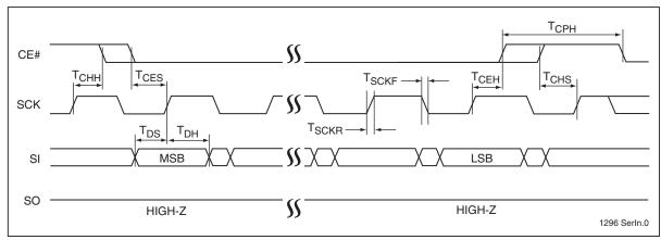
Figure 22: Serial Input Timing Diagram
