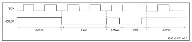
Figure 4: Hold Condition Waveform
