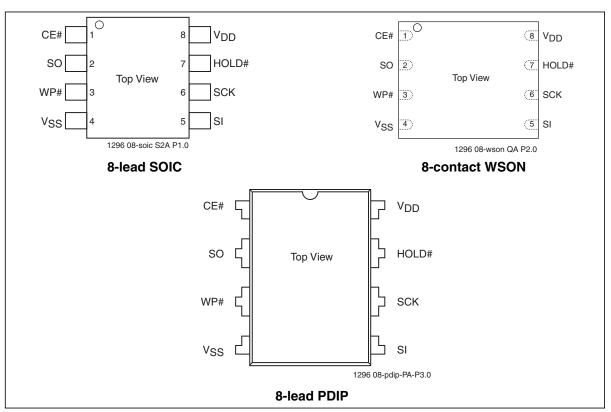
Figure 2: Pin Assignments
