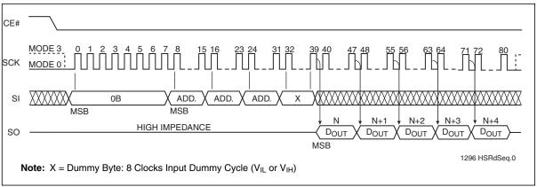
Figure 6: High-Speed-Read Sequence
