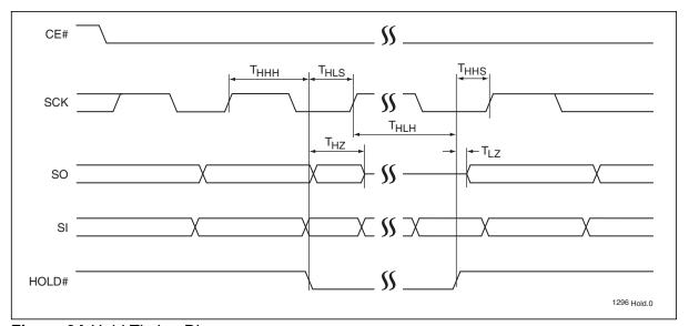
Figure 24:Hold Timing Diagram
