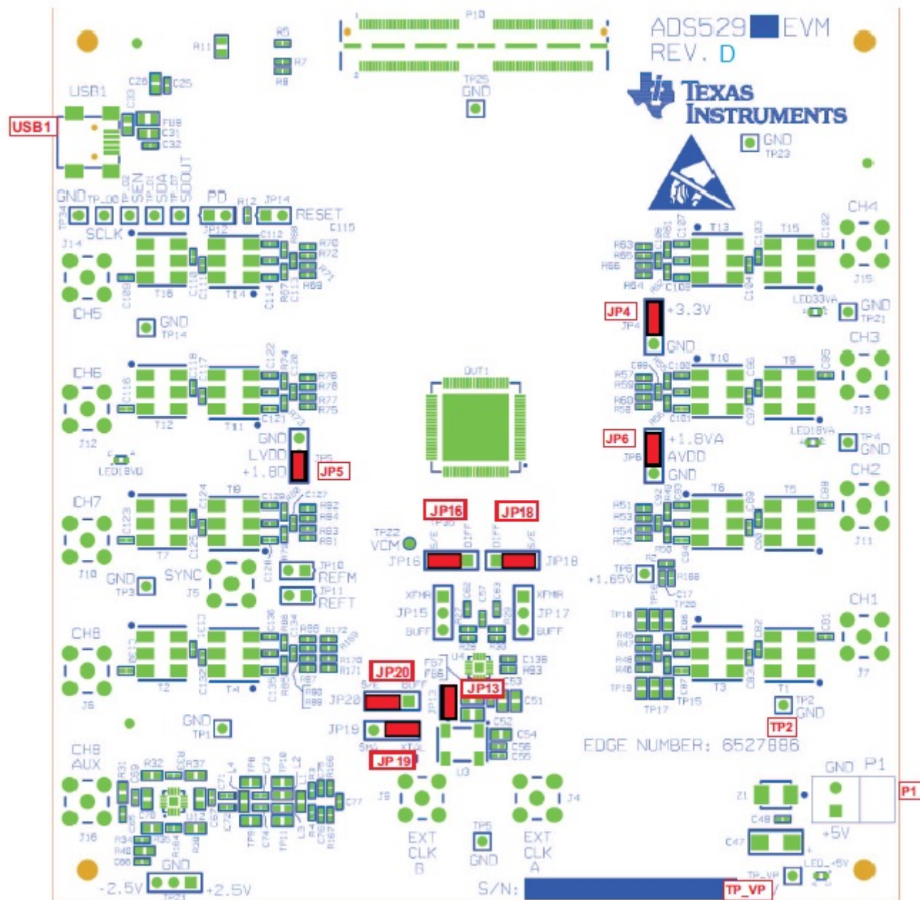
Figure 2. ADS5295EVM Basic Configuration
